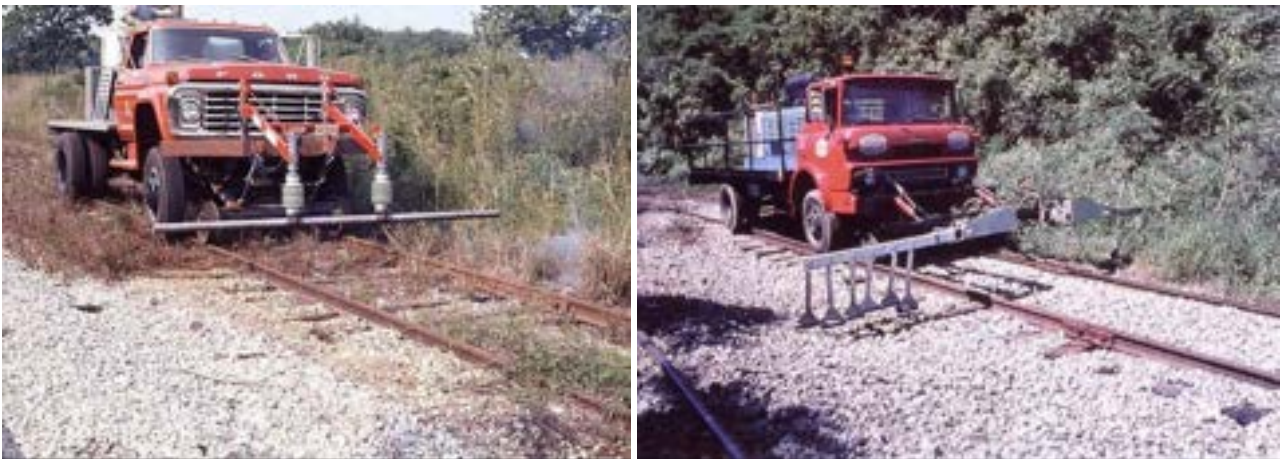
Figure 4. Railway weeding system. Photos Lasco via Dr Mike Diprose.
