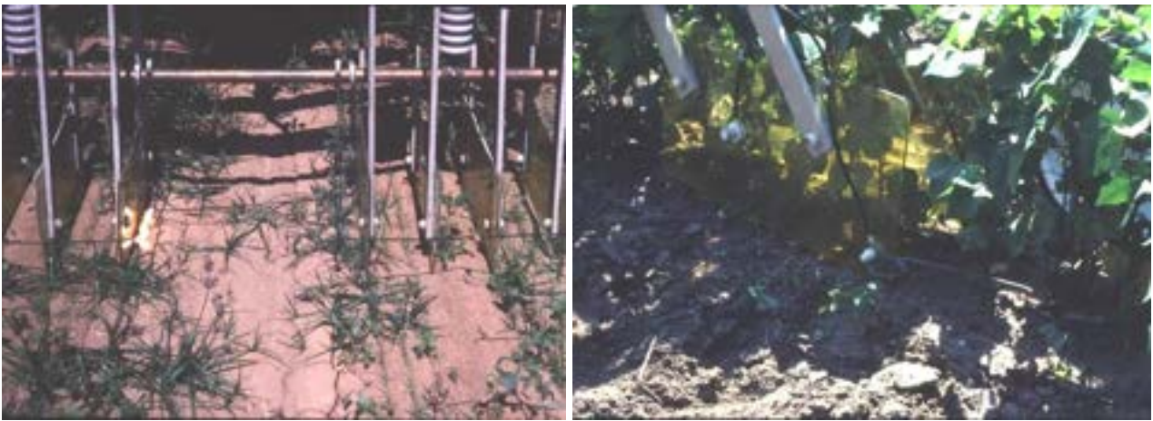
Figure 3. Electrothermal interrow hoe. Photos Lasco via Dr Mike Diprose.
