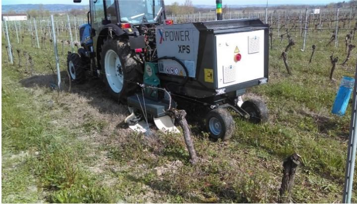
Figure 1: XPS Gen1 equipment with applicator mounted at the back, using a New Holland T4 tractor, at a speed of 2.5 km/h and 3.5 km/h. 6 x 3KVA power units (no power boost used). Soil moisture: 5 to 25%. Soil type: clay-loam.
