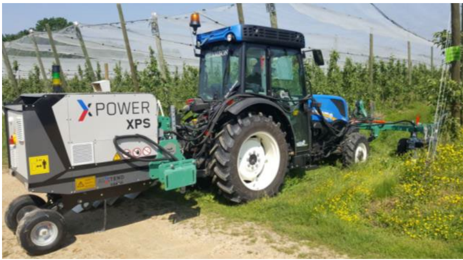
Figure 1.0: XPS Gen1 equipment with applicator mounted on a front frame, using a New Holland T4 tractor, at a speed of 2.5 km/h. 6 3KVA power units. Soil moisture: 5-25%. Soil type: clay-loam.
